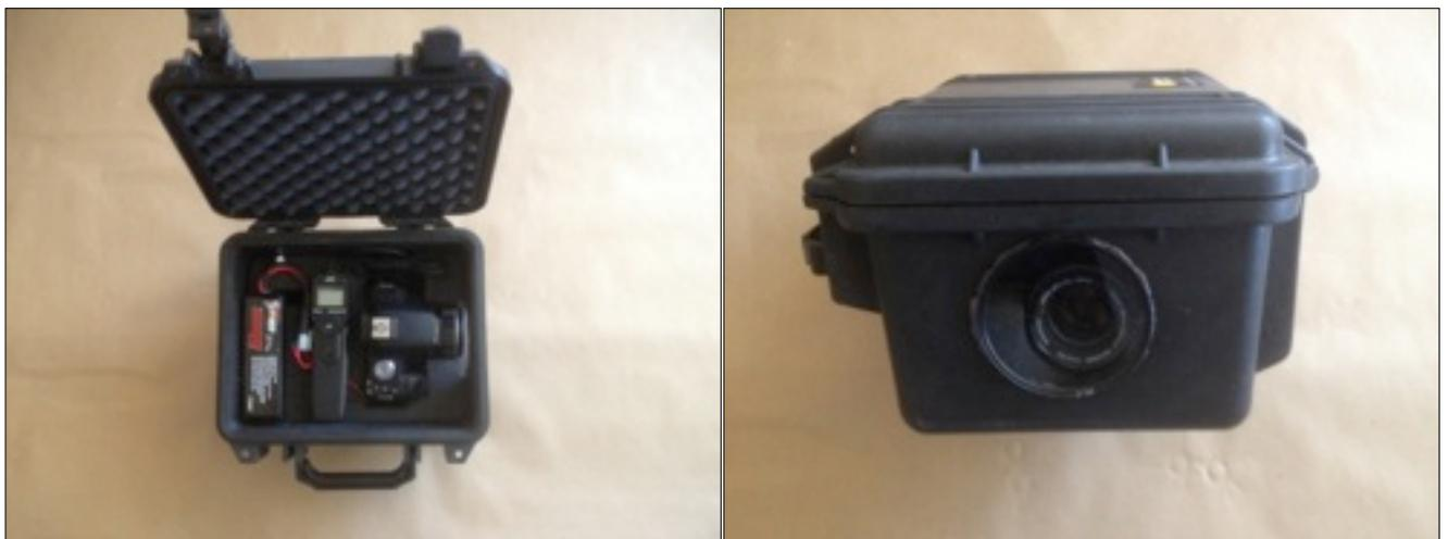
Fig 7. In the pelican case (left) and all closed up (right). Note that you will need to remove and trim the foam inside the pelican case to accommodate the camera and other components.
